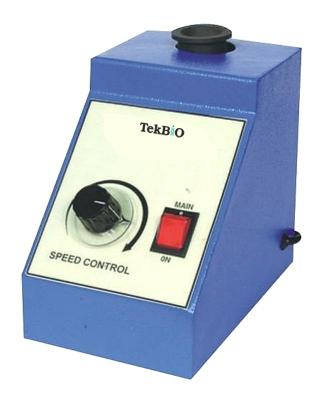
A vortex mixer, or vortexer, is a simple device used commonly in laboratories to mix small vials of liquid. When a test tube or other appropriate container is pressed into the rubber cup (or touched to its edge) the motion is transmitted to the liquid inside and a vortex is created.
